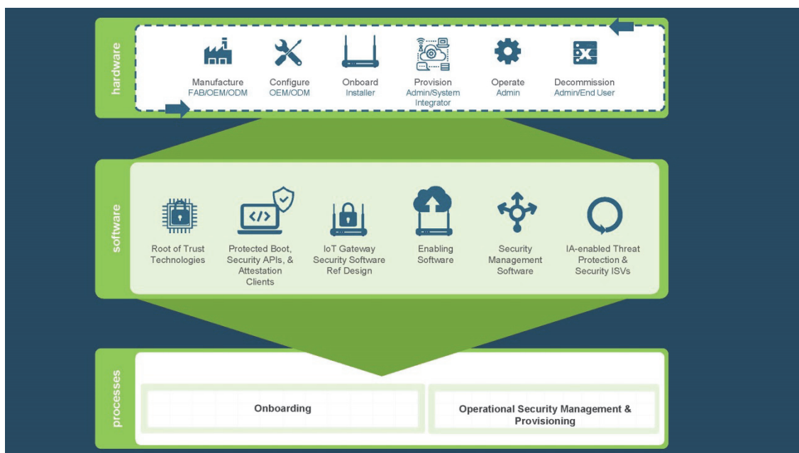
FIGURE 7 EXTENDED RISK-BASED APPROACH: SECURING EVERY DEVICE THROUGHOUT ITS LIFE-CYCLE
